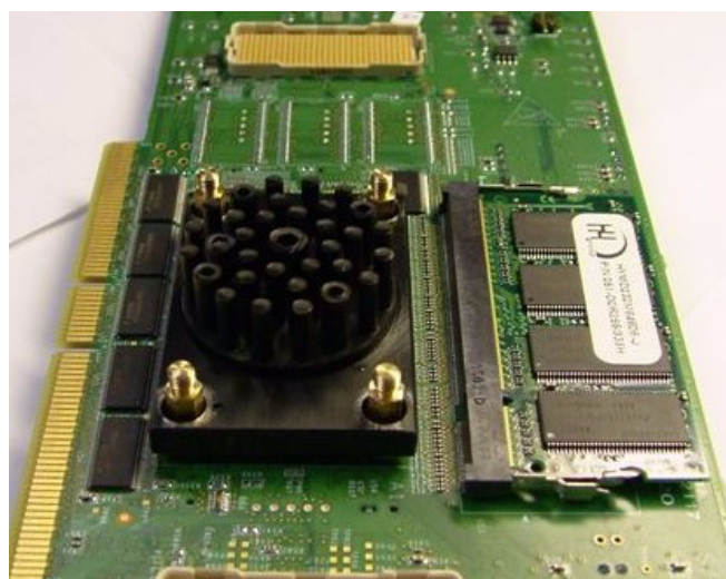
Figure 7-12 Allen screws removed
